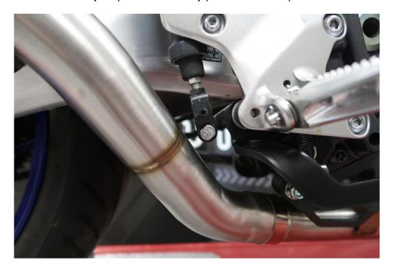
Then using the supplied fixings install the pillion peg mounting bracket - removal of the OE peg mounting pin is required here- then loosely hang your silencer and retain with the mounting bolt finger tight
