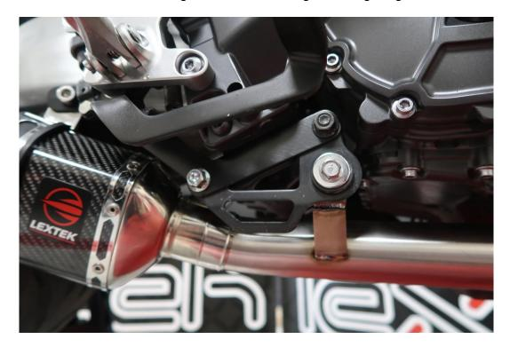
At this point tighten the mounting bracket fixings to 30nm and continue to the final fit section
