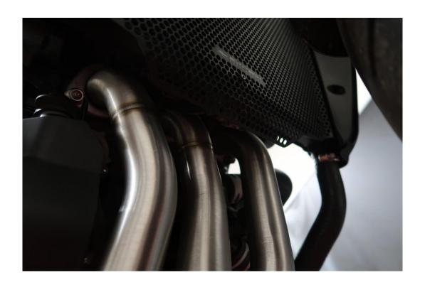
Loosely install the mid pipe mounting bracket bolt and retain with the nut finger tight.
