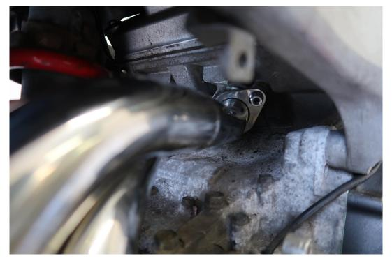
Connect the mid section to the rear down pipes using the springs (supplied).
